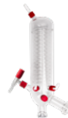
Vertical condenser (steam rises)
