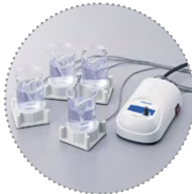
Same speed for all connected stirrers CS-1 and CB-1 controller
