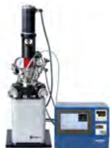
Temperature,Stirring Speed,Cooling Valve Controller
