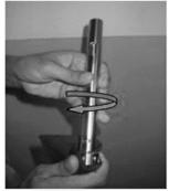
2. While holding the stator, turn the shaft tube clockwise until the stator is loosened inside the shaft tube
