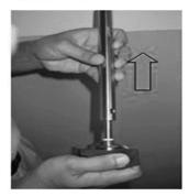
3. Remove the shaft tube and put it at a place where it cannot fall down or otherwise be damaged
