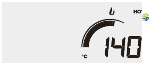
The display now alternates between the set temperature (with dots between figures) and the actual temperature (no dots between figures) every 5 seconds.
