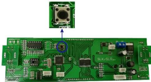
The contact switch on processor board
